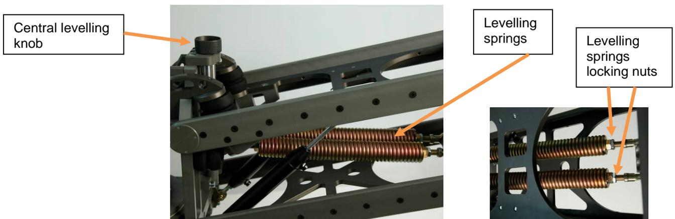
Turning the central levelling knob clockwise will raise the arm, anticlockwise will lower it.
